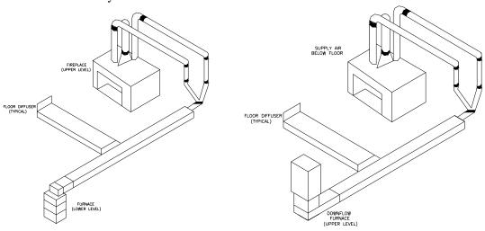
FIGURE 16a: DUCTING SYSTEMS EXAMPLES
